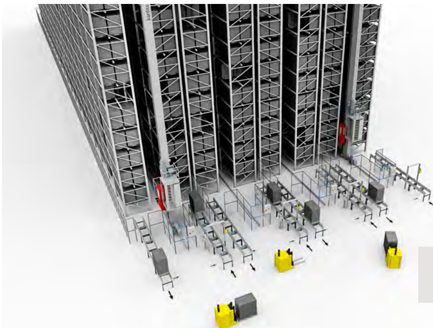
Automated storage and retrieval systems in mixing room
